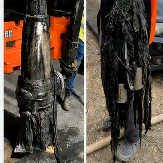
Grease hardened in pipes
