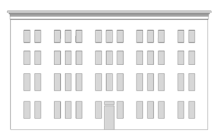
Figure 5-6: A cornice at the top of the mass
