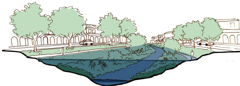
Left: Sketches show how public spaces such as the one shown in the illustrative plan can also serve to help with flood control. Most of the time, the space is green with a low flow channel and can accommodate trails and wildlife habitat (top). In the event of a large storm, the channel is designed to fill and provide expanded flood storage (bottom). The naturalized channel provides for beautiful long views and welcomes people to enjoy the space with trails and nature walks.
