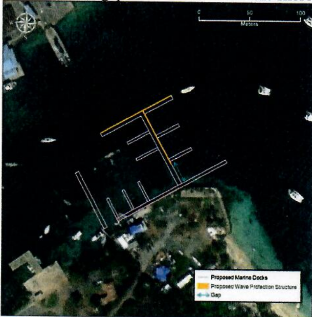
Figure 9.00.1: Proposed Marina Location and Wave Protection Structure (Design Condition) Initially, the design looked to extend the wave barrier perpendicular to the shoreline up to the shoreline in order to provide the maximum protection (Alternative 1). Initial flushing simulation results showed that this would significantly increase the overall flushing times within Vessup Bay. Two other alternatives were run. The first had a gap of 23 feet between the shoreline and the wave protection structure (Alternative 2). The second had a gap of 46 feet (Alternative 3). The runs with a gap of 70 feet was shown to have no negative impact on circulation.
